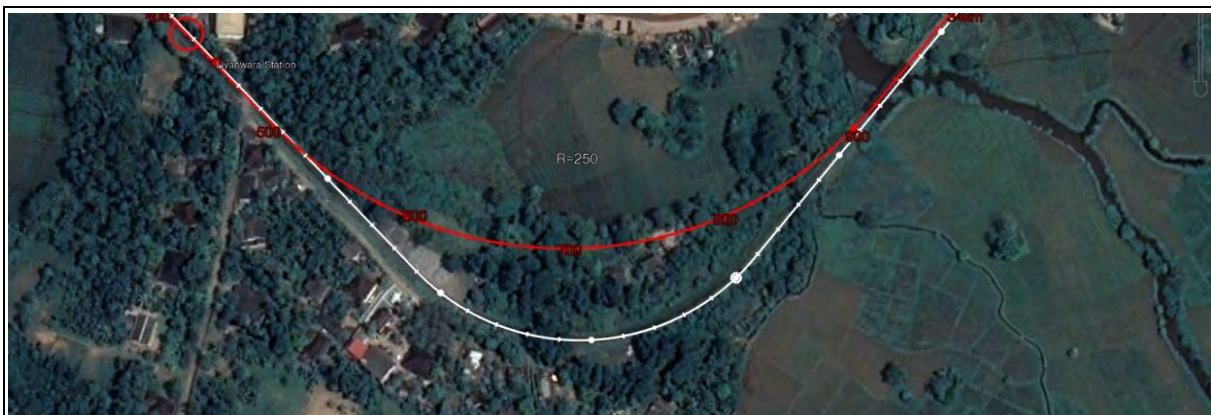
Figure 5-10 27km280 ~ 28km090 : Changing alignment is possible
