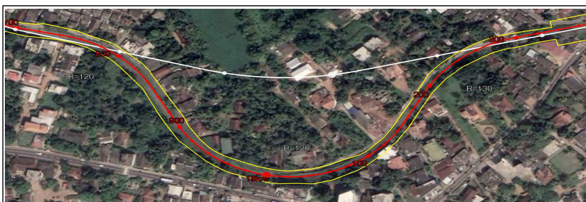
Figure 5-4 14km860 ~ 15km400 : Changing alignment is possible
