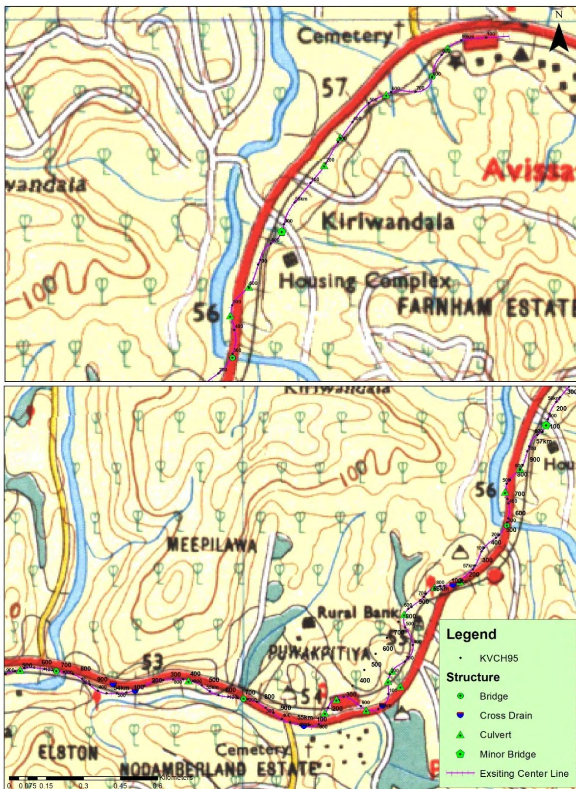
Figure 3-8 Hydraulic Structure Location Map from 44+000km to 53+400km
