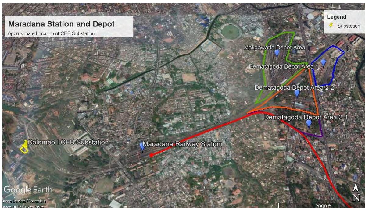
Figure 10-8 Proposed Feeder Stations- Near Maradana Depot
