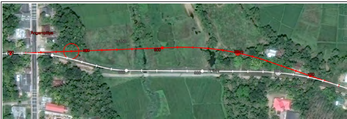
Figure 5-12 36km200 and 36km600 : Changing alignment is possible
