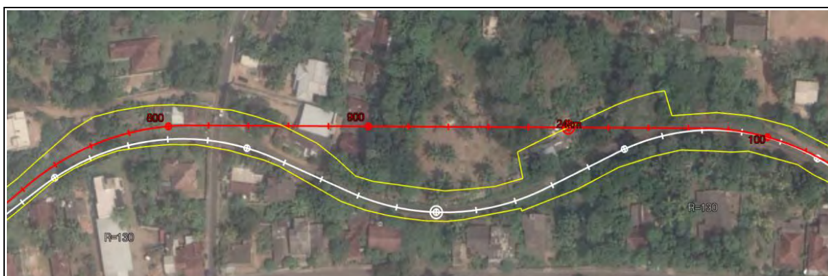
Figure 5-7 22km600 ~ 22km800 : Changing alignment is possible
