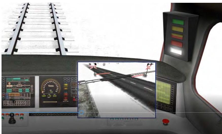
Figure 12-26 Driver's Cab Level Crossing CCTV Display (Prom-Electronica, 2007)
